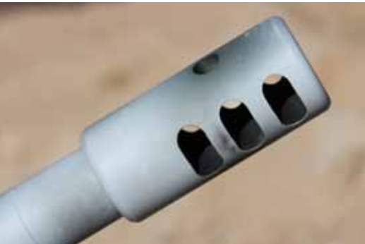
D&L Sports' muzzle brake has two side ports and one on top. Recoil was negligible and no dust kicked up from the ground when firing from the prone position.
